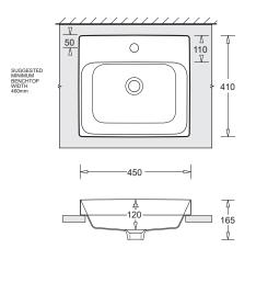
BASIN MAY BE SEALED TO COUNTER TOP USING ACETIC CURE SILICONE SEALANT II USE EPOXY ADHESIVES
